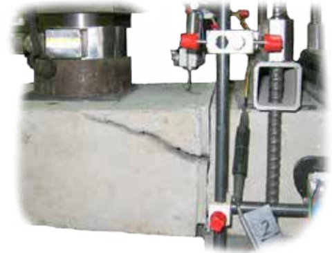
Typical "pop-out" failure of tested dowel system
